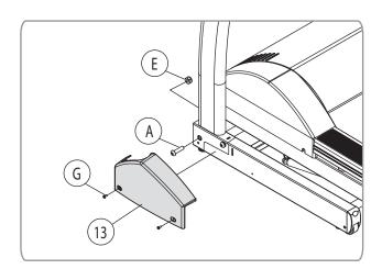
C. Attach the left (13) and right (14) base covers using a Phillips screwdriver and 2 machine screws (G) on each side. The 4 base cover attaching screws are located in the hardware bag.
